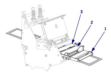
**8.** Push the media forward until it passes under the printhead assembly (1), under the snap plate (2), and then over the platen roller (3).
